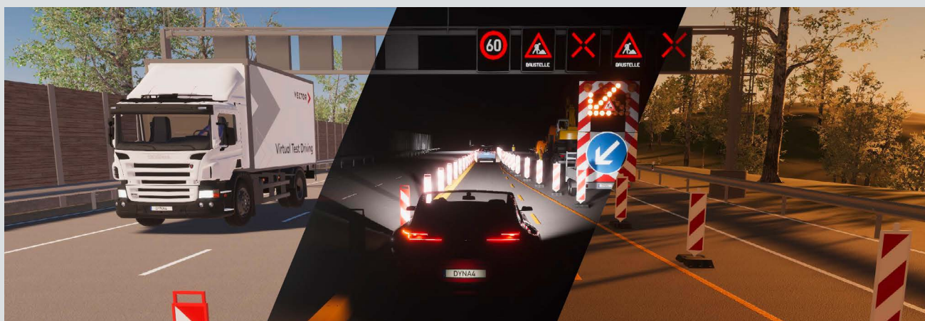
DYNA4: Test driving in a virtual environment with different light conditions
